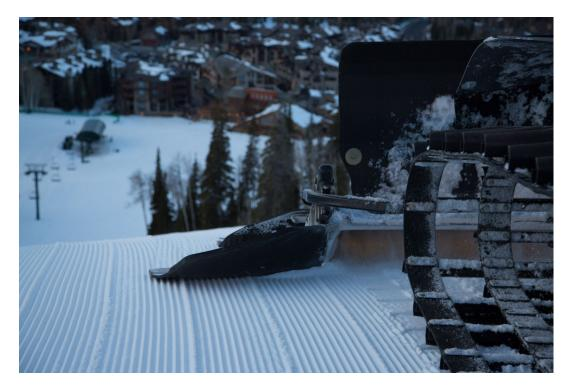
The first objective is to loosen compacted snow and start driving it back up the hill. Steeper runs and obstacles like moguls require a winch cable – measuring almost 4,000 feet long – the aid in this fight against gravity by offering improved traction. Hard and compact conditions offer another set of challenges. By nature, there is less snow available to loosen, either by skier or cat, then move back uphill in the blade.
